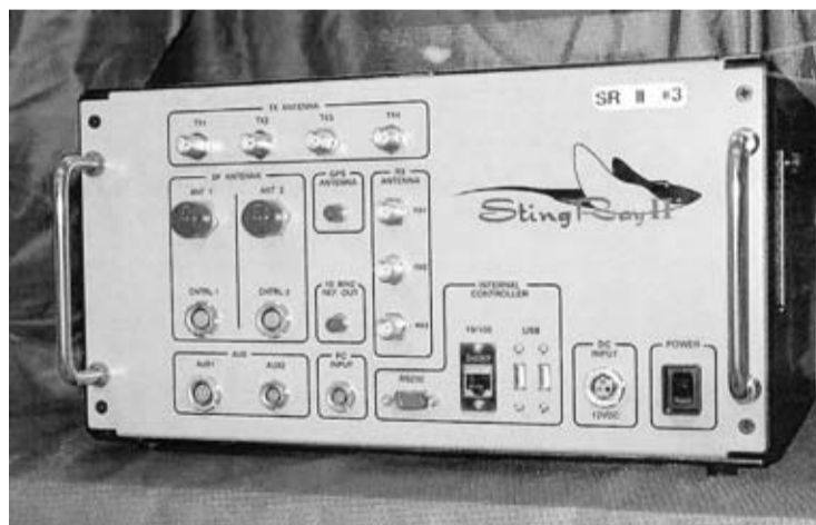
This undated file photo provided by the U.S. Patent and Trademark Office shows the StingRay II , a cellular site simulator used for surveillance purposes manufactured by Harris Corporation, of Melbourne, Fla.
